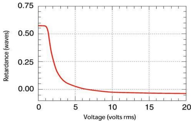
**Figure 1 – Shows the change in retardance with voltage for a typical LCVR.**
