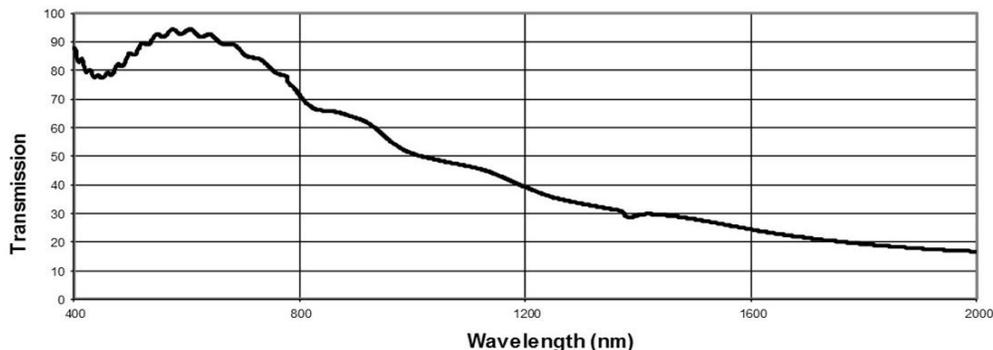
**Figure 3 – Shows the measured open state transmission of a TN LC cell that has not been antireflection coated.**
