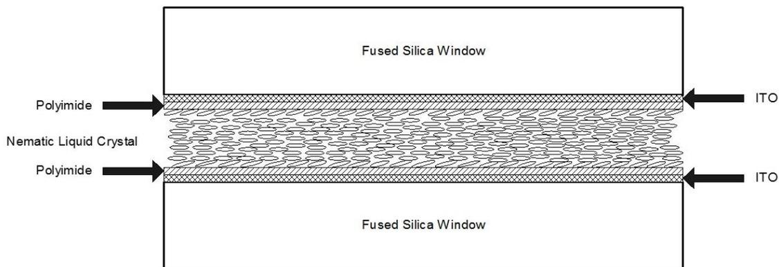
**Figure 2 – shows schematically the structure of a nematic LCVR.**
